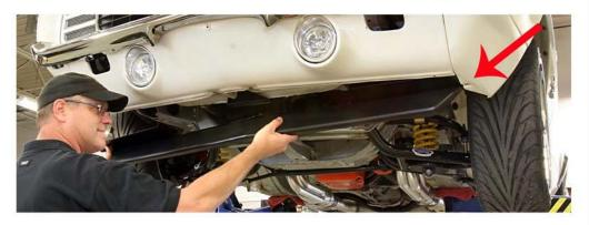
Slide one end of Bottom Feed plate into a fender/ valence opening (position kit as shown). Front edge of the main plate should be above the rearward lip of the front lower valence panel.
