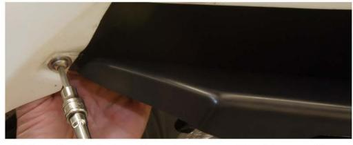
Using the bolts/washers/nuts provided in small plastic bag, insert bolts upward through the holes at ends of kit plate & the lower corners of the fenders. Tighten with 5/32 inch Allen socket/6 inch ext/3/8 inch ratchet & 1/2 inch wrench.
