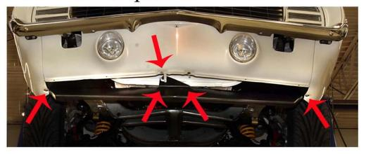
Go back over all of the fasteners and tighten everything to 104 in-lbs. Now the Bottom Feed kit is installed and ready for action.
