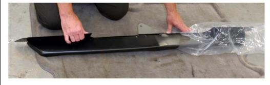
Find a large pad to work on to minimize scratching of part—in this case, we used a floor pad out of an SUV. Then, pull the Bottom Feed kit out of the protective shipping bag & set it on the pad.
