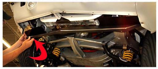
Swing other end of kit rearward about 6 inches before setting on lip of the other fender & valence panel. Keep leading edge of main plate above rear edge of front lower valence panel. Kit will be resting on the lower lip of front valence & fenders.
