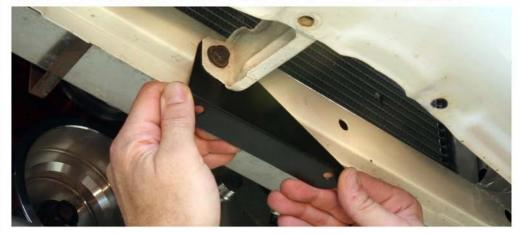
The bracket needs to be lightly pushed forward so the 'L' bracket for the Bottom Feed kit can be slid in between the bracket and core support, as shown. Hand start the factory bolt back in the threaded hole and tighten it to hand tight.
