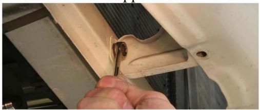
Using the 1/2 inch wrench, remove the center bolt on the lower lip of the radiator core support. This bolt holds a factory bracket that comes off the
