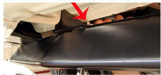
One at a time, push ¼ inch diameter stainless 'L' bracket bolt & washer combo up thru hole in main plate & 'L' bracket. Hand start nylock nut on the bolt. Tighten with 9/64 Allen socket on 6 inch ext & 3/8 inch ratchet wrench & 7/16 inch wrench.
