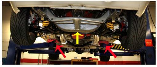
Some vehicles sit too low to install the kit—if so, vehicle should be raised in the front (lift with floor-jack on crossmember – at yellow arrow) & placed on two jackstands (locate at red arrows). If another spoiler on the vehicle, remove it at this time.
