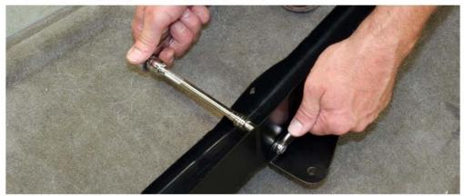
The center 'L' bracket needs to be removed to install the kit. Use 5/32 inch Allen socket/6 inch ext/3/8 inch ratchet wrench & 7/16 inch wrench to remove both bolt/nut combos.
